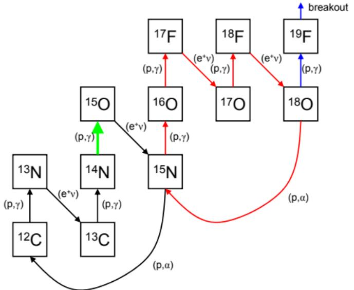
$^{14}\text{N}(p, \gamma)^{15}\text{O}$ : slowest step, determines rate
