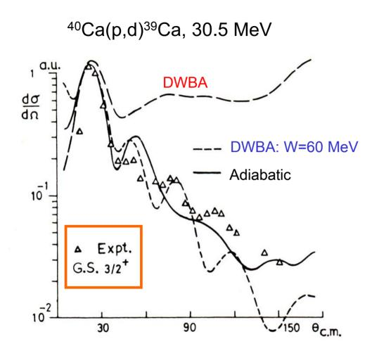
Increased reflection at nuclear surface - less diffuse deuteron channel potential
