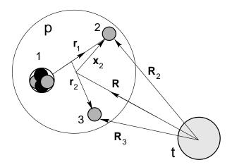
FIG.1 Definition of the coordinate vectors used in the case of a three-body projectile.
