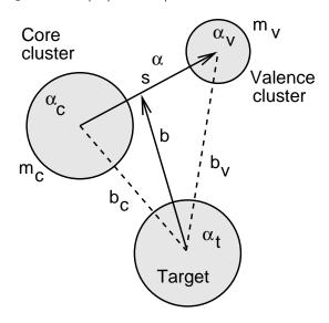
FIG.5 The two-cluster projectile coordinates relative to the target. The co-ordinate z-axis, the projectile beam direction, is directed into the page.
