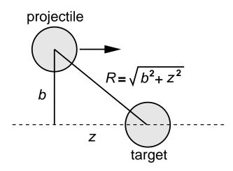
FIG.3 The straight line trajectory assumption of the eikonal approximation.
