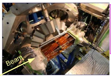
Active silicon stopper array: 5 DSSSDs, 1 mm thick 60x40 strips, each 1 mm wide Spacing: 0.5 mm
